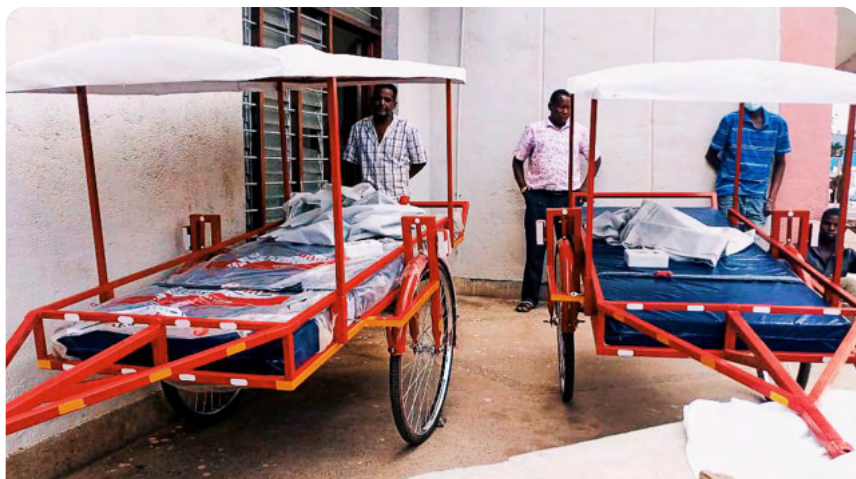
Malawi: Ambu-bikes being built to increase access for maternal patients to healthcare facilities
